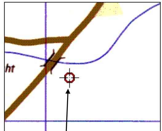
If the bridge's location is measured precisely (e.g., GPS receiver), the bridge might really be located as shown by the target icon. There is a significant offset of the target icon from the bridge icon on the map. Because a very accurate location is required for a GPS-guided bomb to hit the bridge, a map display might show two separate locations for the same bridge.
