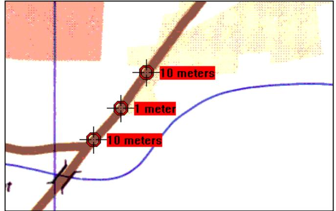
In the figure at right, the accuracy of each collection asset is again noted next to each vehicle icon. This time two collection assets are relatively inaccurate. This suggests that the three icons represent two or more vehicles.
